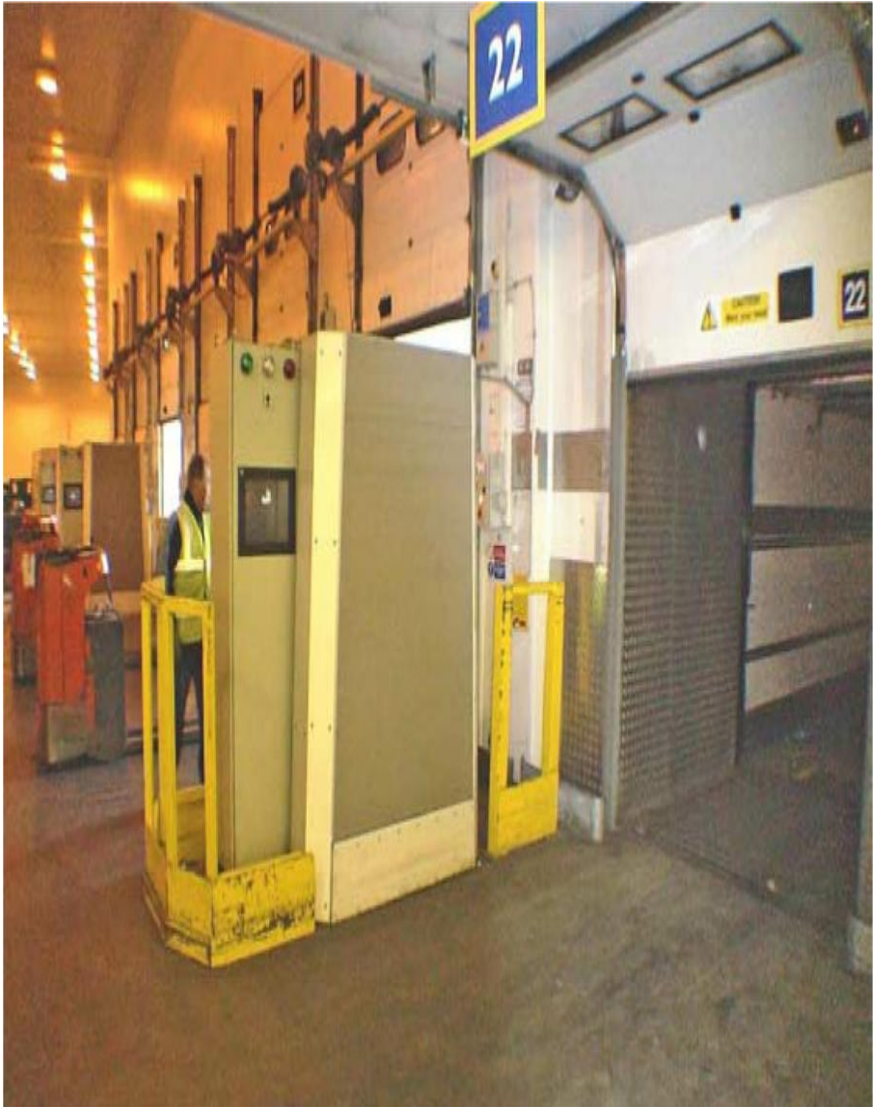
Figure 10.22 RFID tags for tote tracking at Marks & Spencer.
