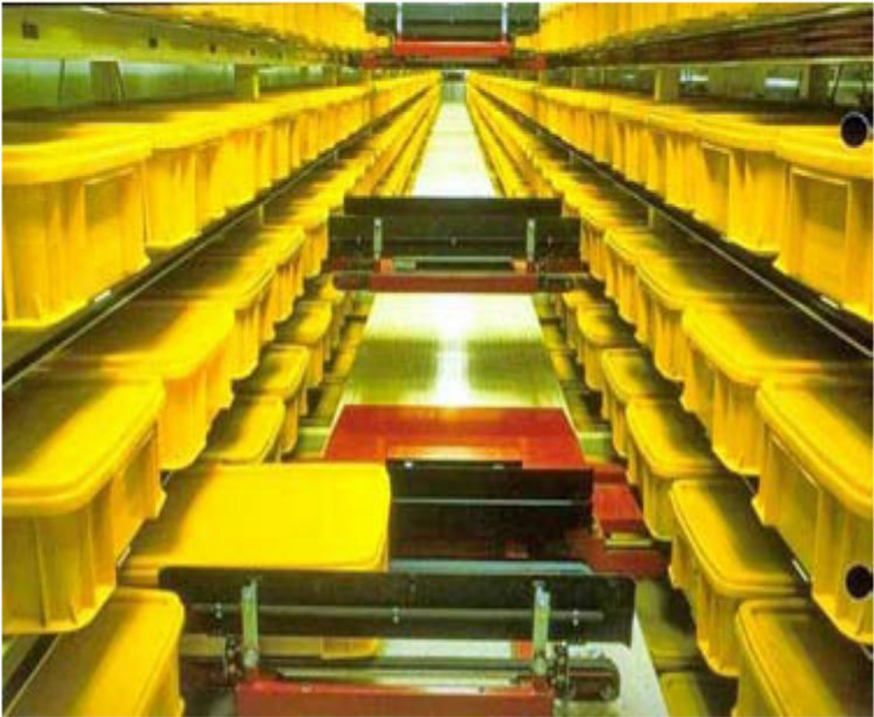
Figure 7.55 Miniload ASRS for mining maintenance parts.
