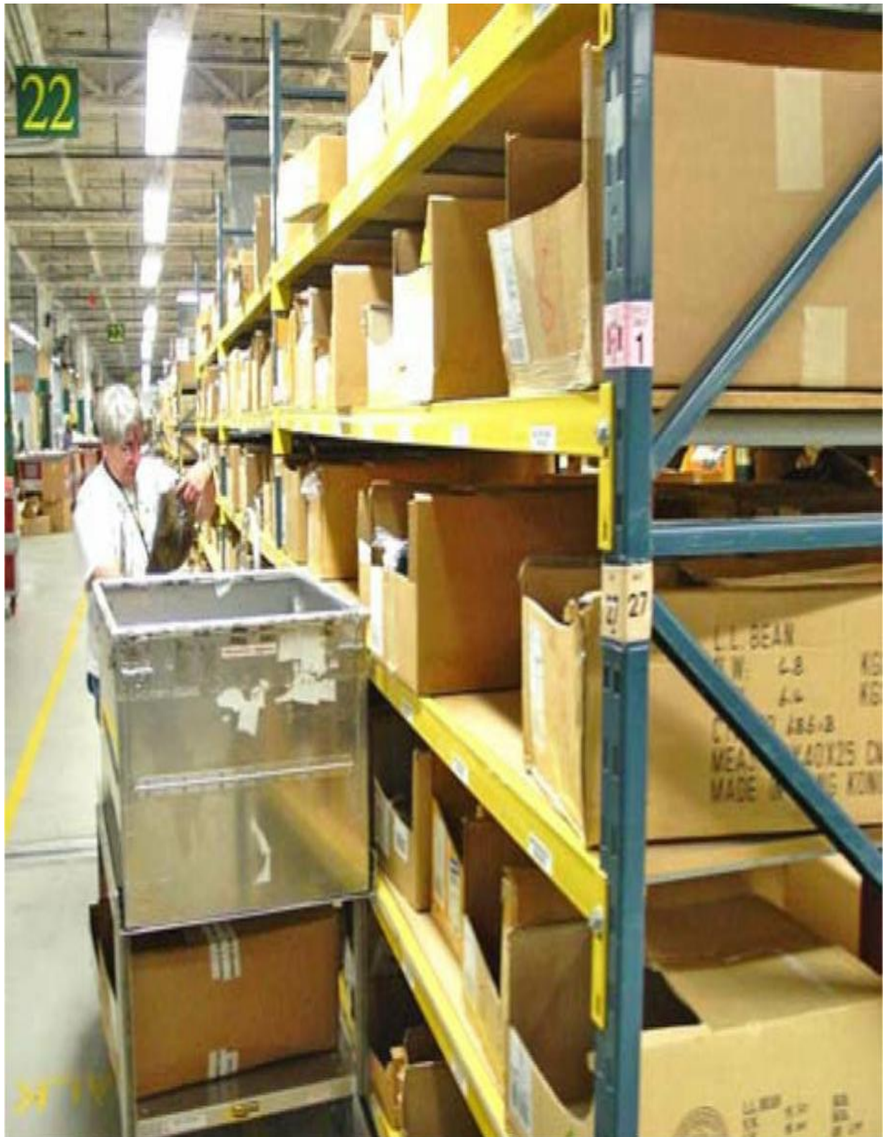
Figure 7.32 Batch wave picking cart releasing poly-bagged garments into
