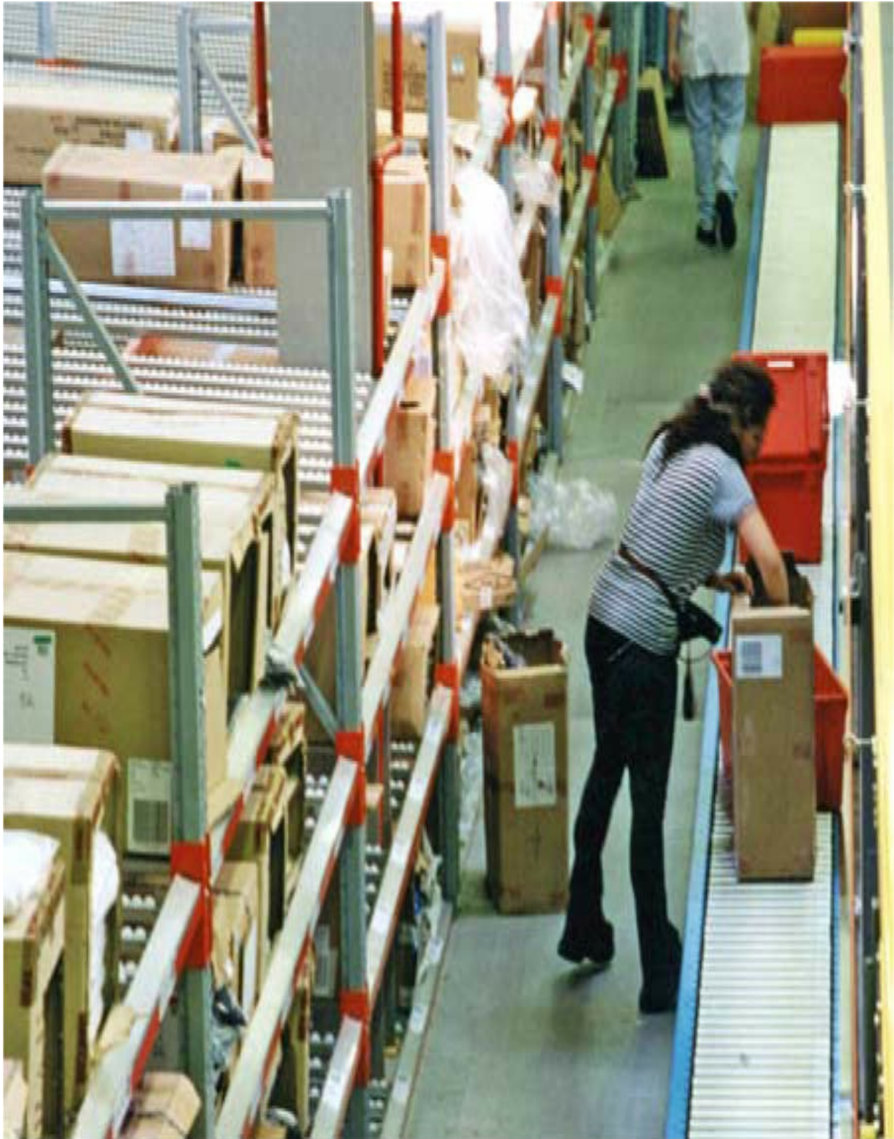
Figure 7.18 Carton flow-rack pick-to-light.
