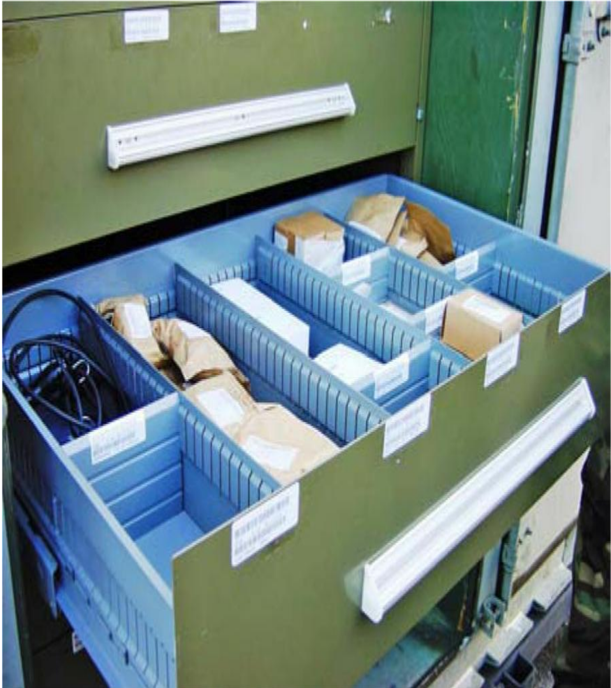
Figure 7.11 Typical storage drawer configuration (Lista).
