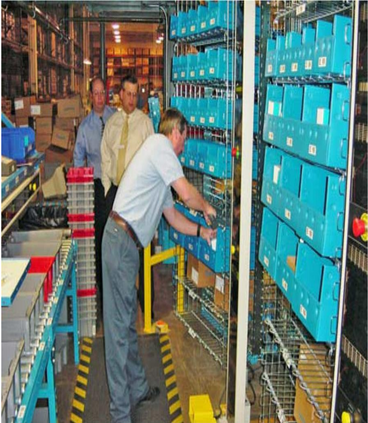
Figure 7.45 Horizontal carousel system with automated outfeed and loop front end at Witt.
