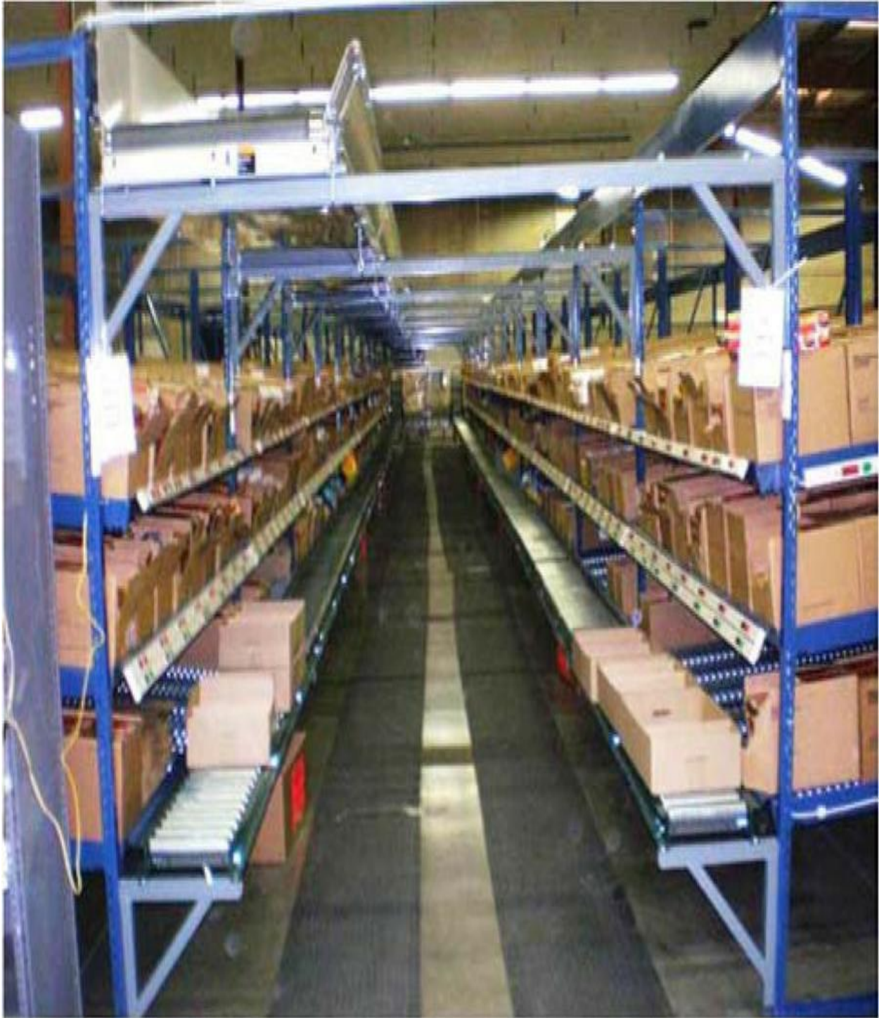
Figure 10.38 Pick-by-light and put-by-light to retail-store totes aided by next-pick and next-put director and motion detector to prevent mispicks and misputs (AT&C).
