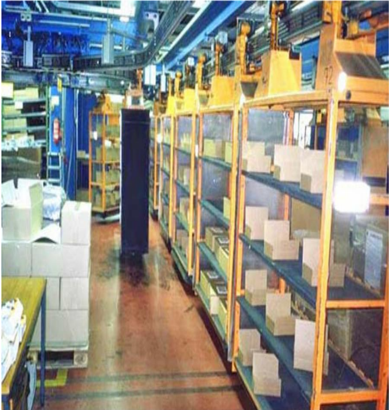
Figure 7.28 Batch picking cart equipped with onboard scales, onboard labeling, and onboard computing.
