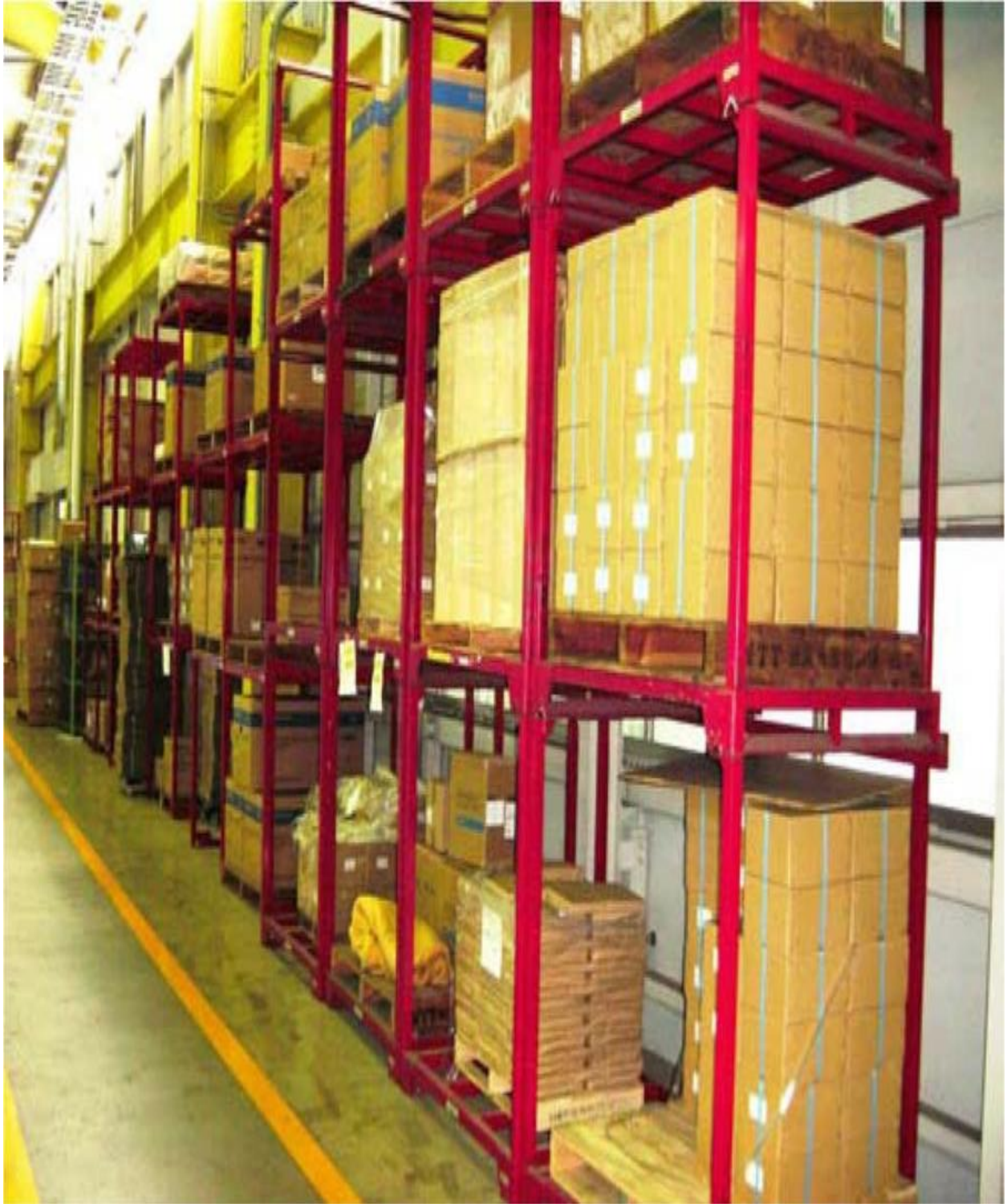
Figure 5.11 Inbound pallet stacking frames arriving to a Ford warehouse Georgia.
