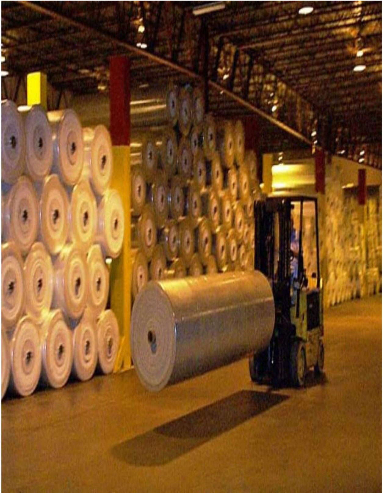
Figure 5.32 Stand-up counterbalance lift truck at NTT (Tokyo, Japan).
