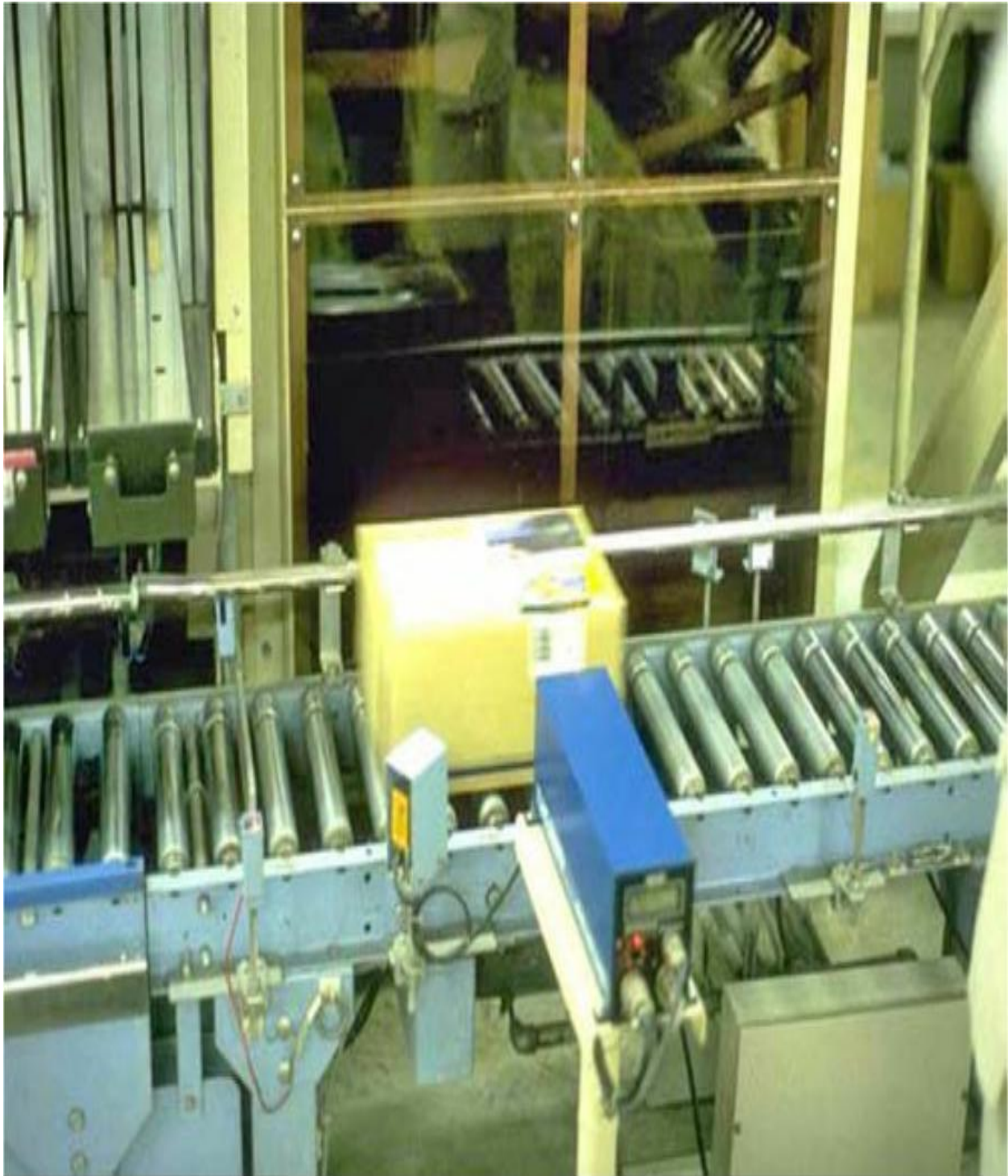
Figure 10.17 Omnidirectional bar-code scanning.
