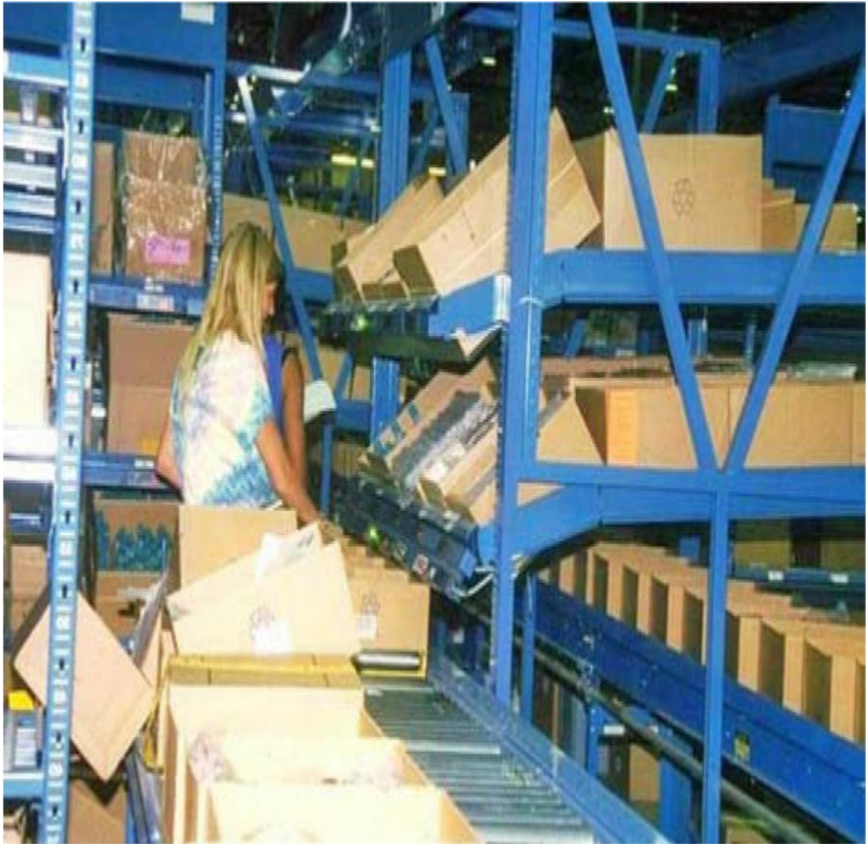
Figure 7.20 Carton-flow-rack simulation for Avon.
