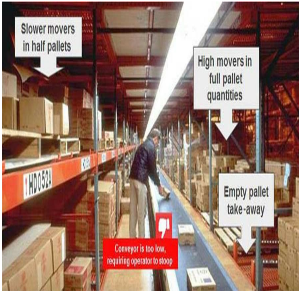
Figure 6.20 Case pick to belt at a BIC finished goods distribution center.
