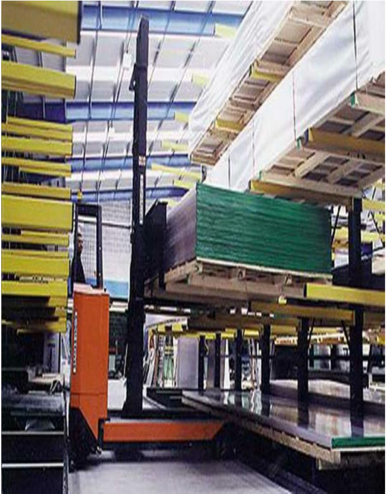
A typical aisle would be 6½ feet wide, rail or wire-guided. Side loaders
