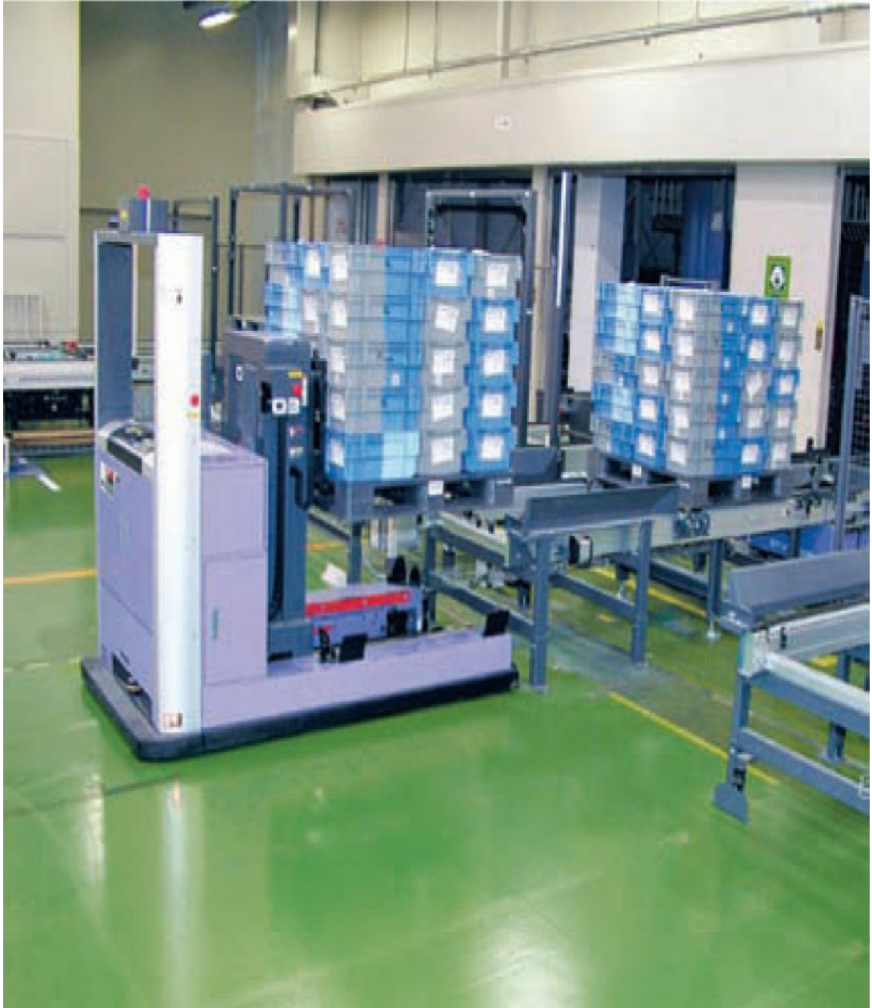
Figure 9.15 Small-load autonomous mobile transporter (Adept).
