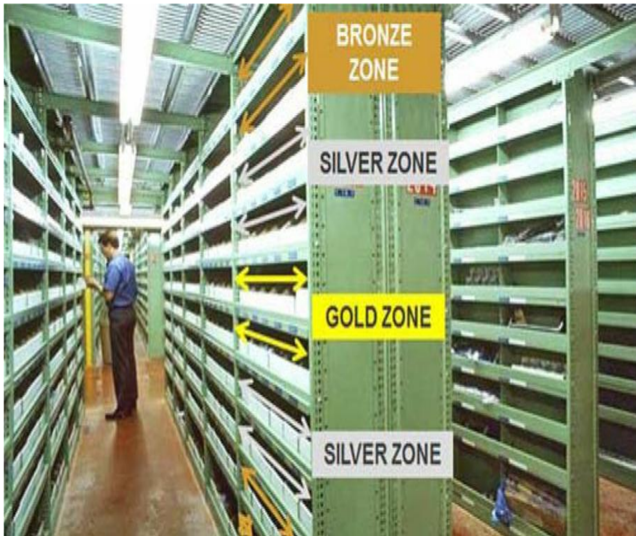
Figure 7.3 Bin shelving system with corrugated inserts for small-parts picking.
