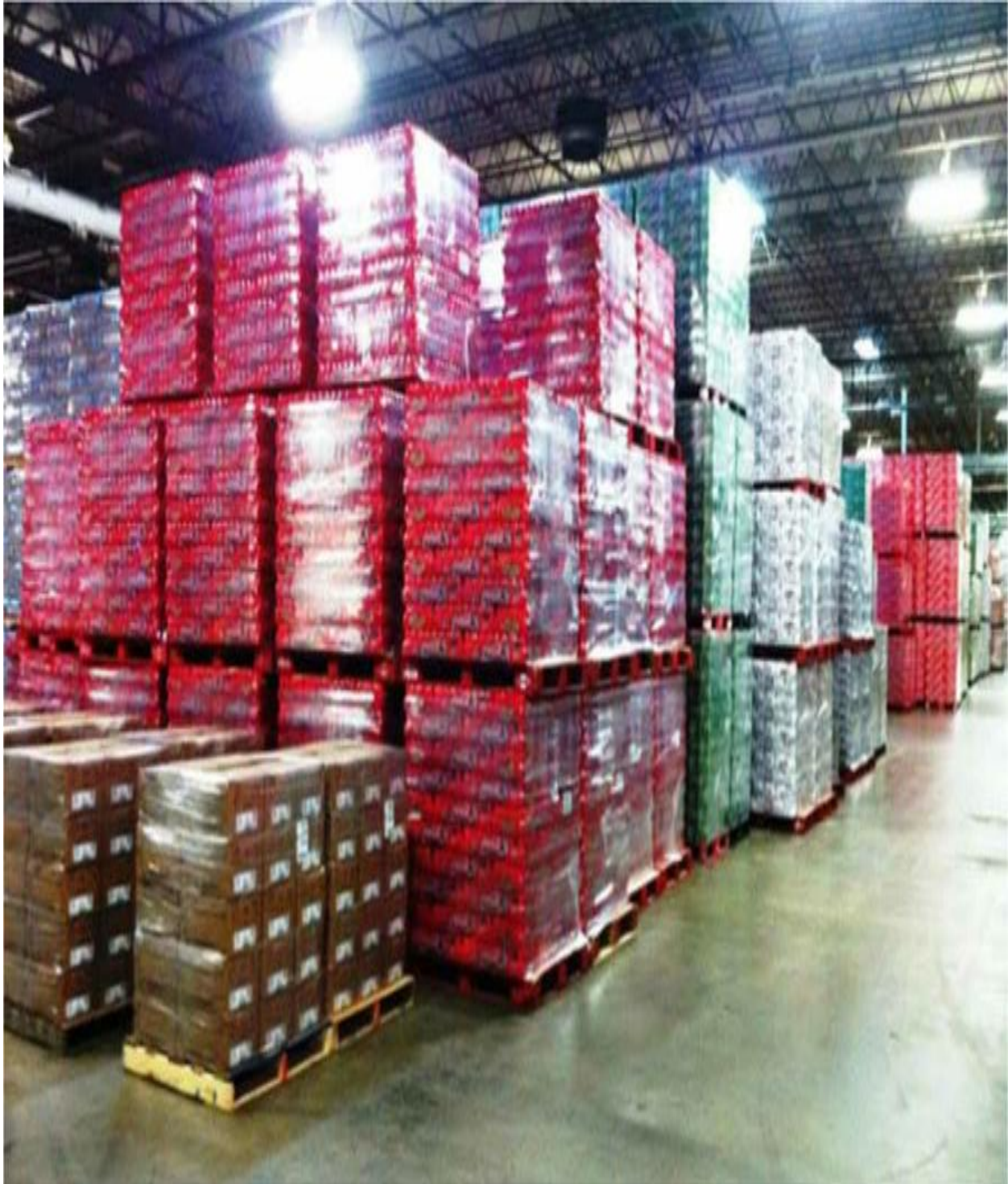
Figure 5.3 Floor storage may be the only reasonable pallet storage alternative in a warehouse with low clearings. Such was the case at this Japanese beverage wholesaler's multi-story distribution center.
