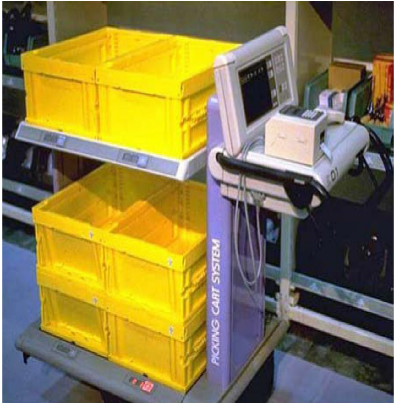
Figure 7.34 Automated guided vehicle (AGV) picking cart. (Creform)
