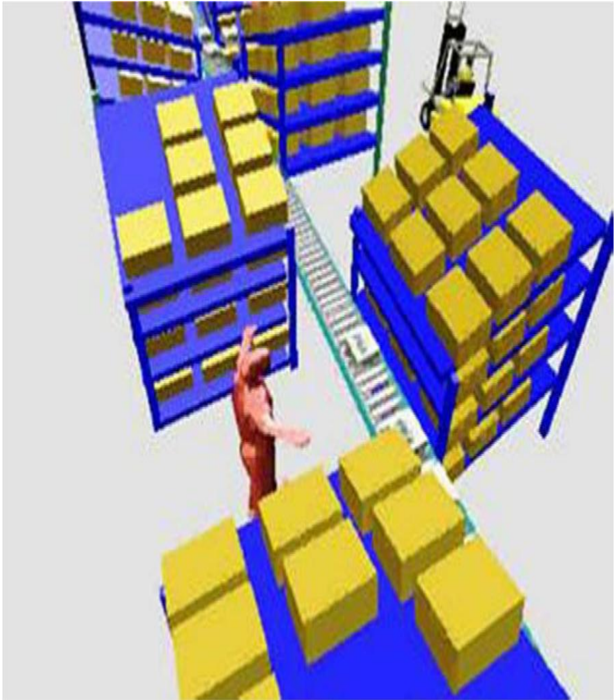
Figure 7.21 Carton-flow-rack bays at L.L. Bean.
