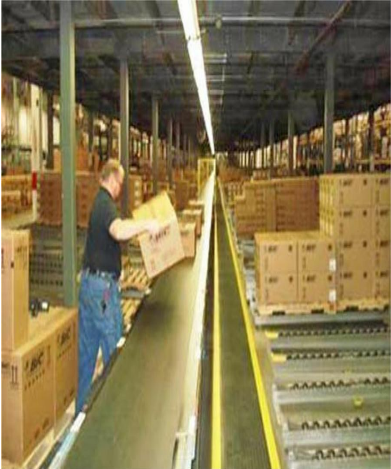
Figure 6.21 Case pick-to-conveyor at Verizon's East Coast distribution center.
