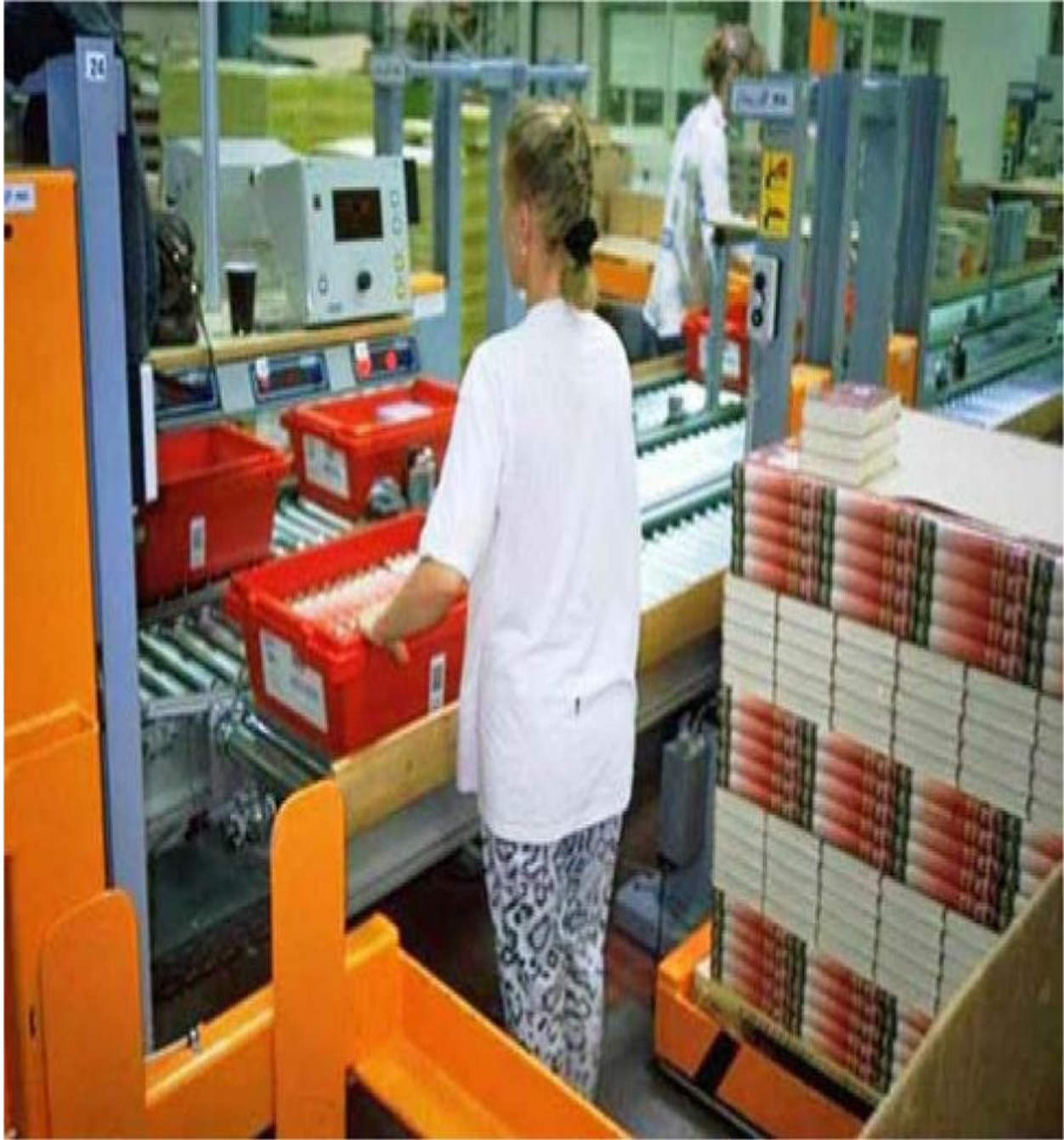
Figure 10.32 Pick-to-light with next task director display at Bertlesmann (Gutersloh, Germany).
