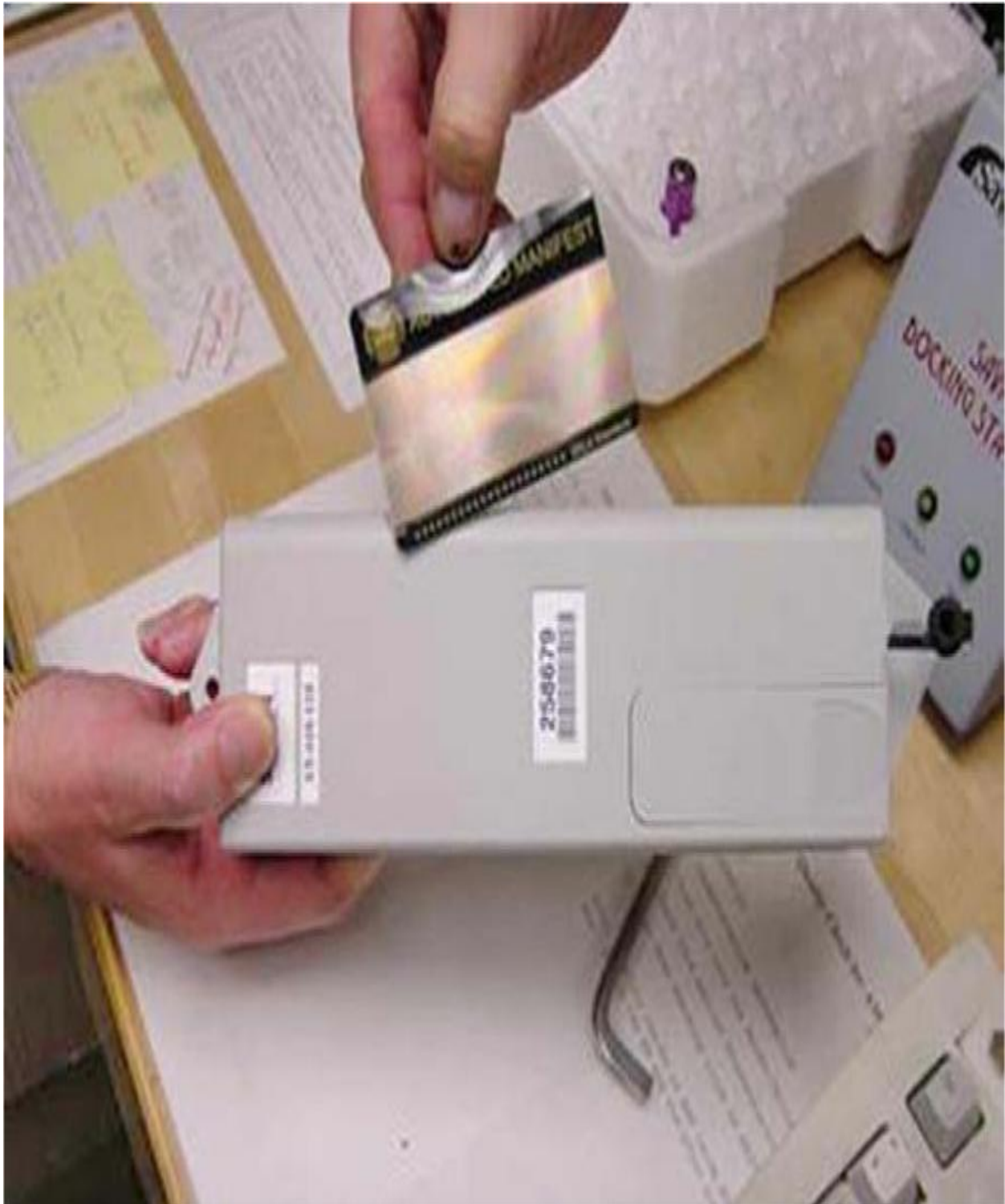
Figure 10.26 Smart cards used in an order-picking application at Shiseido's Tokyo distribution center. Each card's magnetic stripe holds a picking tour. The smart cards are read by a smart card reader attached
