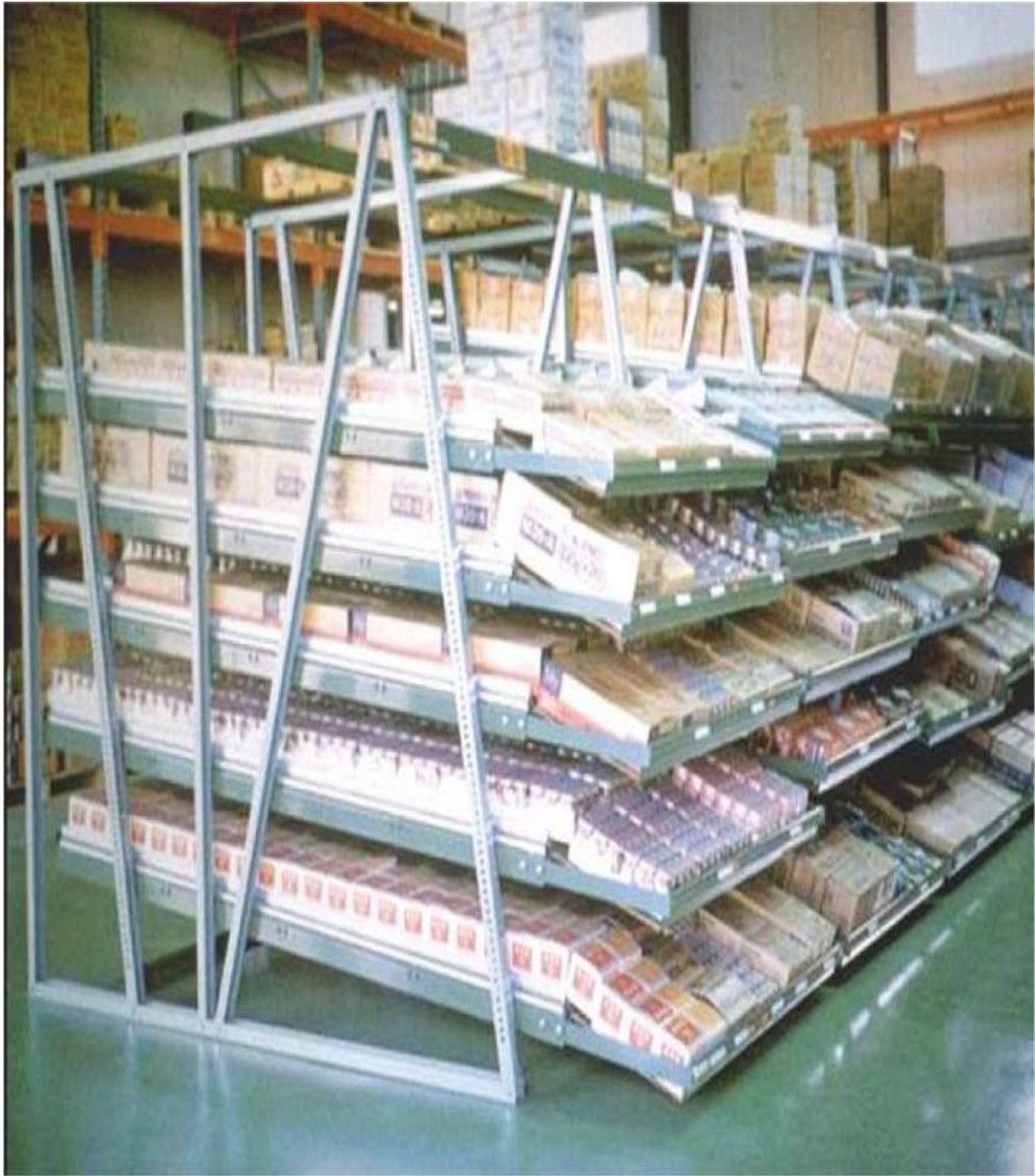
Figure 7.16 Carton-flow-rack picking line at NTT's Tokyo logistics center.
